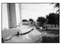
DH Tech can use different sources for power including electric, gas (propane or natural) and steam in order to run the dehumidifier in a more economical way for the customer. Here, propane is used as a power source.
